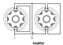
Series-Parallel wiring two dual 2 ohm subs = 2 ohm
