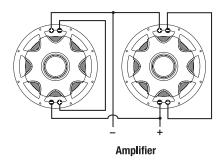
Series-Parallel wiring two dual 4 ohm subs = 4 ohm
