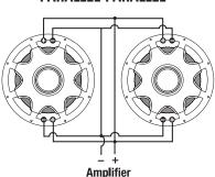
Parallel-Parallel wiring two dual 4 ohm subs = 1 ohm
